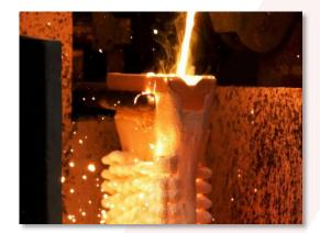
Investment Casting is synonymous with creators of products which have dimensional accuracy, a must feature for investment casting, in which castings of complex designs are needed. Since every used wax pattern is destroyed after use, a large number of such wax patterns are needed and Atul Precision Cast does not have quantity production as an obstacle. In fact, the large-scale production makes them cost-effective in an expensive technology.
